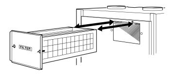
The heat pump's air filter needs to be cleaned regularly (approximately 4 - 5 times per year). The interval between cleaning operations varies and depends on the amount of dust in the exhaust air.
