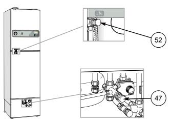
FIGHTER 360P has two safety valves, one for the heating system and one for the water heater.
